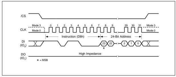
Figure 17. Block Erase Instruction Sequence Diagram
