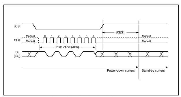
Figure 20. Release Power-down Instruction Sequence
