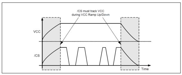
Figure 26b. Power-up, Power-Down Requirement
