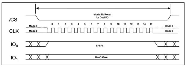
Figure 13. Continuous Read Mode Reset for Fast Read Dual I/O
