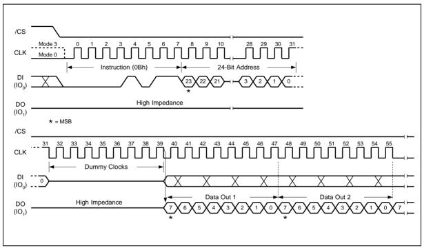
Figure 10. Fast Read Instruction Sequence Diagram
