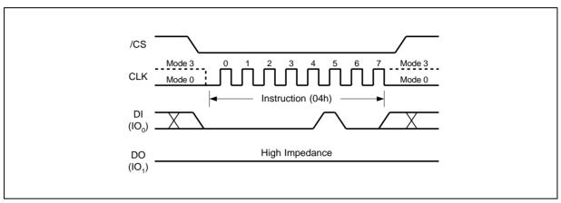
Figure 6. Write Disable Instruction Sequence Diagram
