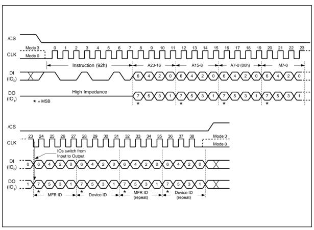
Figure 23. Read Manufacturer / Device ID Dual I/O Diagram
