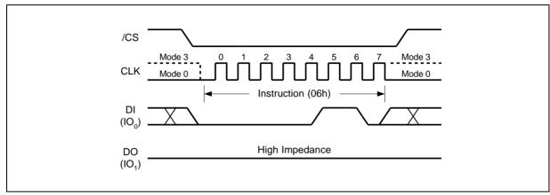
Figure 4. Write Enable Instruction Sequence Diagram
