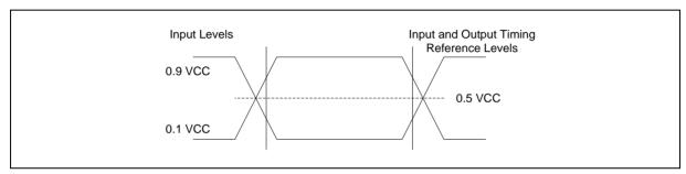
Figure 27. AC Measurement I/O Waveform
