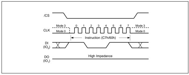
Figure 18. Chip Erase Instruction Sequence Diagram
