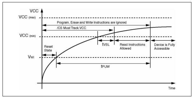
Figure 26a. Power-up Timing and Voltage Levels
