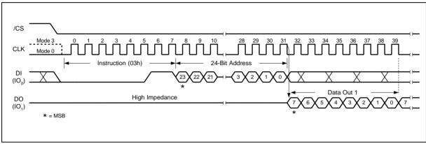
Figure 9. Read Data Instruction Sequence Diagram
