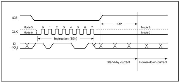
Figure 19. Deep Power-down Instruction Sequence Diagram
